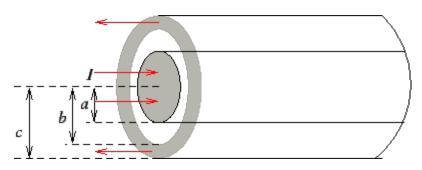
A current I goes into the inner conductor and is returned by the outer shell. Assume the current densities to be uniform both in the shell and in the inner conductor. Calculate magnetic field everywhere.
